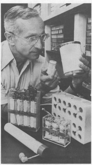
IT'S EASY FOR Sam Levy (2853) to come up with a collection of power packs with the Labs' award-winning TA-23 glass in their cells. Here, the basic 3-volt lithium sulfur dioxide D-cell — in Sam's right hand — as it's used in different Sandia applications.
